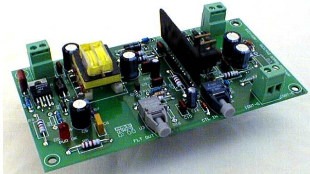
The BAP1318 provides a complete, tested, fast time-to-market solution for companies that need to control and interface to ***High Voltage IGBT*** modules.
